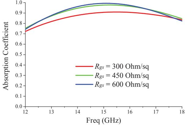
Fig. 4. The absorption coefficients under different value of  $R_{gs}$ .
