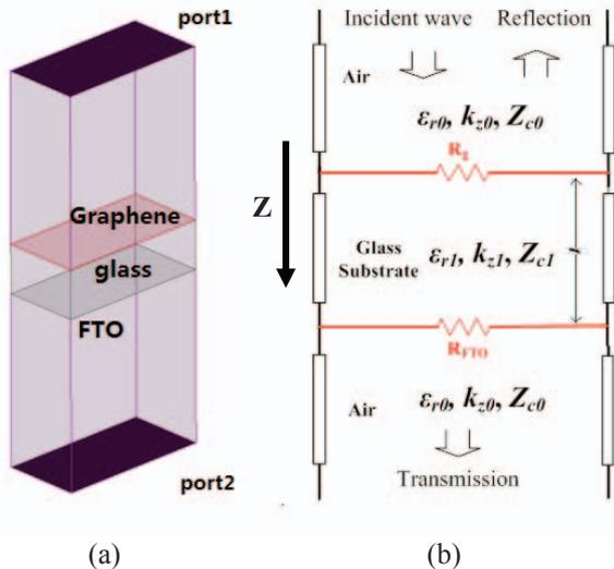
Fig. 2. (a) The model of 3-D full wave simulation and (b) its equivalent circuit.
