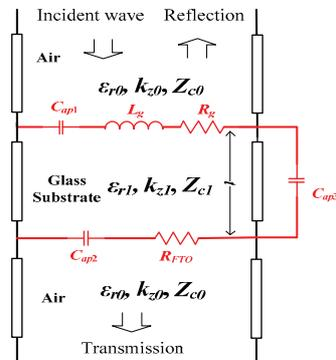
Fig. 6. The improved equivalent circuit model.
