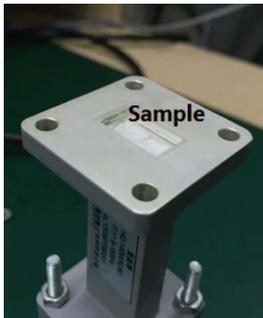
Fig. 5. The placement of the sample in the waveguide.
