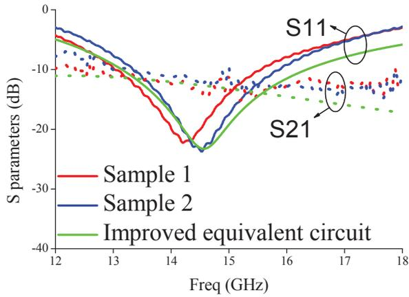
Fig. 7. The scattering parameters of measurement and improved equivalent model.
