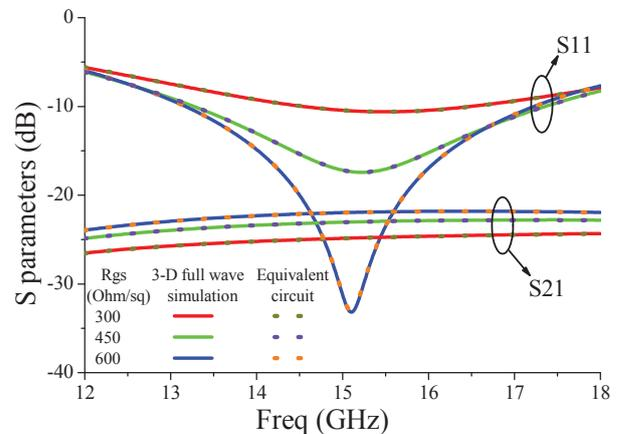
Fig. 3. The scattering parameters calculated by using 3-D full wave simulation and equivalent circuit.
